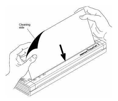
FIGURE 17. Inserting the cleaning cloth
